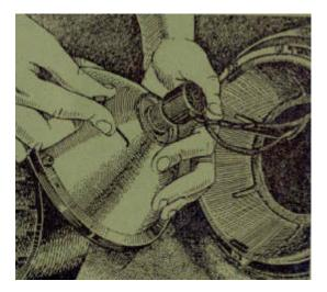
REPLACING THE BULBS IN THE INNER LIGHTING UNITS The bulbs are accessible after the shade has been removed by pulling it outwards
